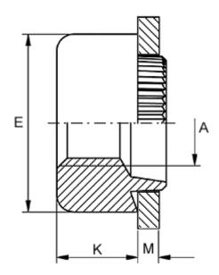
Female thread A = M2Height K = 3.0Outer diameter E = 8.0Plate thickness = 3.5 to 3.7
